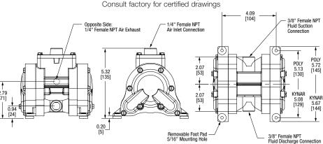
Measurements in inches (millimeters)
